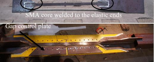
(b) FSBRB penetrated welded core and gap control plates
